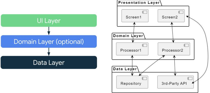
variant: allowing non-adjacent layers to communicate directly (may improve efficiency at the cost of lower readability)
