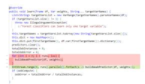
Fig. 2: Example of replace loop with pipeline code upgrade, from padreati/rapaio commit 6d086a1d.
